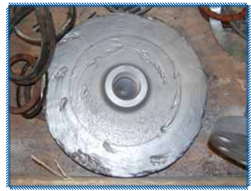
Equipment coming in for repair, above, shows pitting and wear from the abrasive setting in which it operates.
