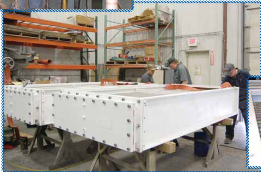
To the left, one of Brimhall's workers fabricates a heat exchanger tube sheet for Hoover Dam. Tolerances are critical. The heat exchanger tube sheet must be precisely aligned for each cut. Below left and right, air coolers for Hoover Dam are reconditioned. These air coolers work on the same principal as a car radiator, just on a much larger scale.
